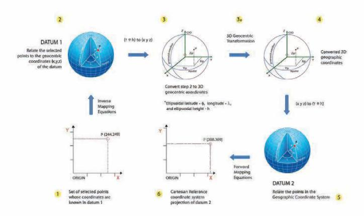
Map and GIS users encounter transformation from one two-dimensional coordinate system to another. This includes the transformation of polar coordinates into Cartesian map coordinates or the transformation from the 2D Cartesian (x, y) system of a particular map projection to another 2D Cartesian (x, y) system of a specified map projection.
